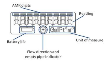
**AMR Digit Bar** (4 to 8 Digits): The AMR digit bar shows which digits will be reported when the meter is read through the communications interface.
